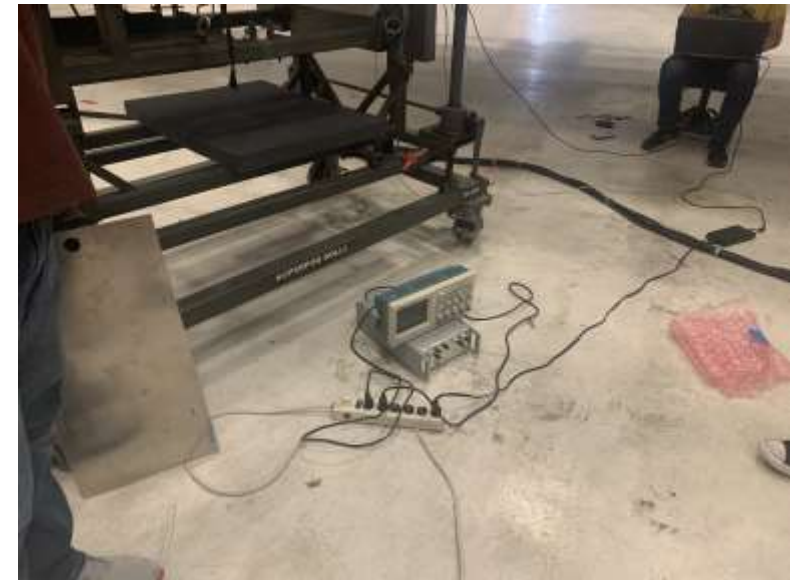
Signal generator and aluminum plate used in the field to debug potential hardware problems on the optical payload.
